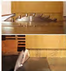
Tenons. Set your saw blade height as shown, then use your miter gauge to cut the tenons.
